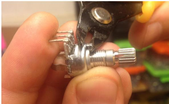
Cut the locating lug on the pot with snips as pictured. Now place the potentiometer on the PCB but... **don't solder it yet!**
