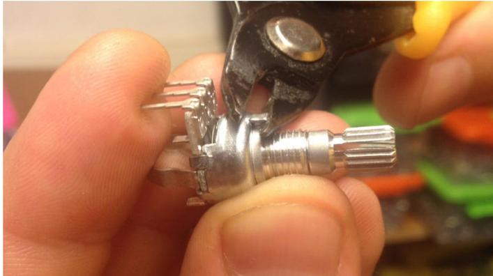
Cut the locating lug on the pot with snips as pictured. Now place the potentiometer on the PCB but... **don't solder it yet!**
